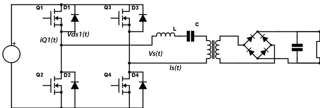
*Resonant techniques reduce component stress and reduce losses incurred by older architecture*
